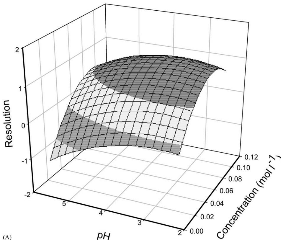
Fig. 2. A, Response surface of resolution, estimated from the central composite design plotted for pH vs. buffer concentration while keeping voltage constant at its central value; B, Contour plot.
