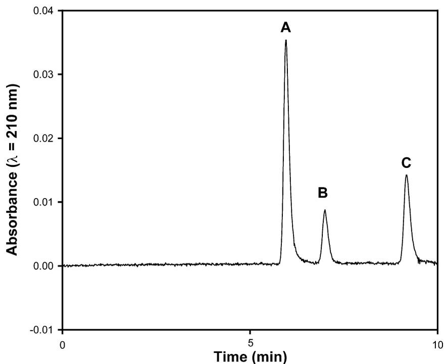
Fig. 1. Electropherogram of a sample containing the three components: A, NAPH; B, PHE and C, DIP, using a buffer phosphate solution of 0.063 mol l<sup>-1</sup>, pH 3.72 and a voltage of 17.7 kV.
